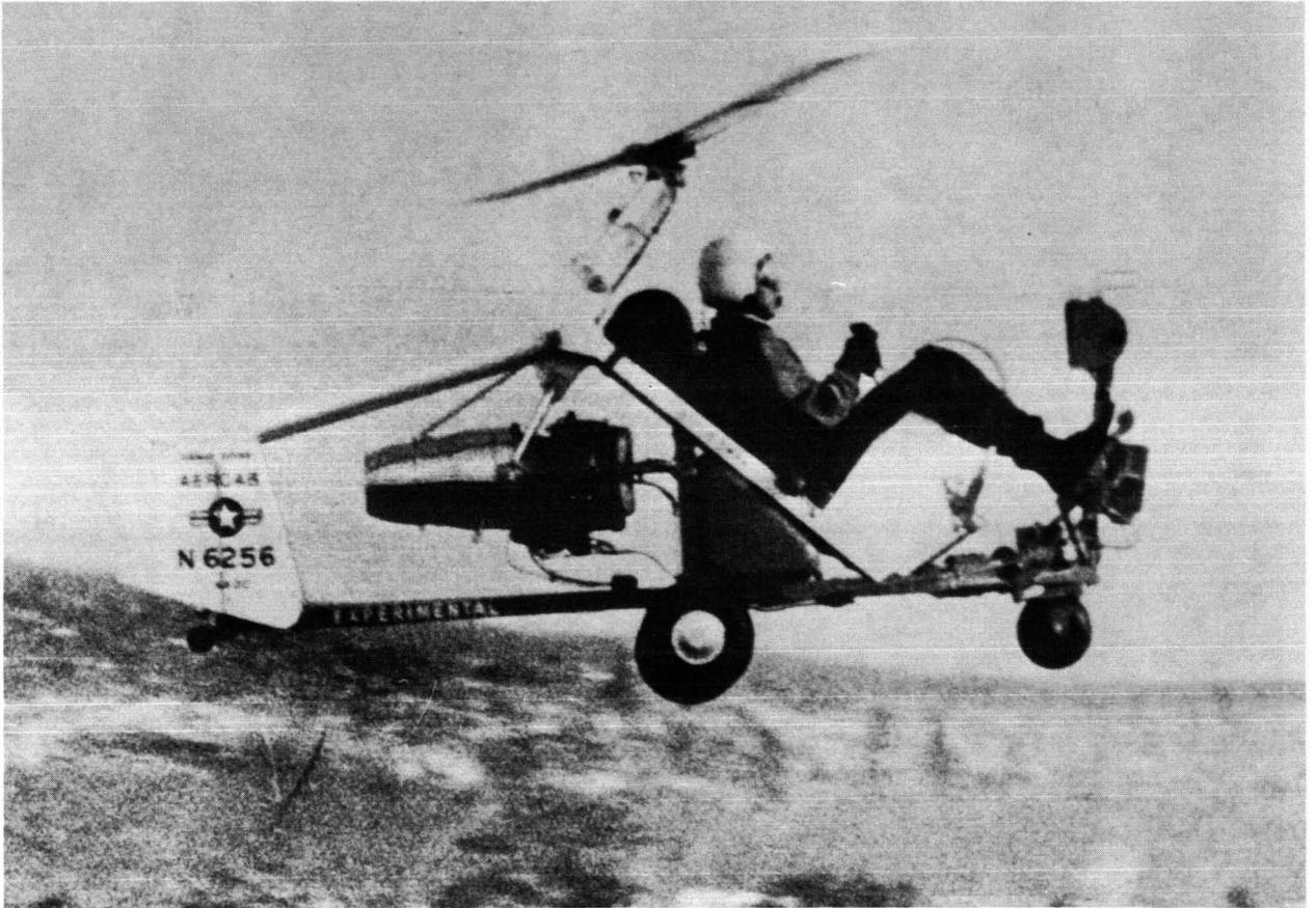
Figure 6. - Autogyro-mode manned flight of the SAVER.
