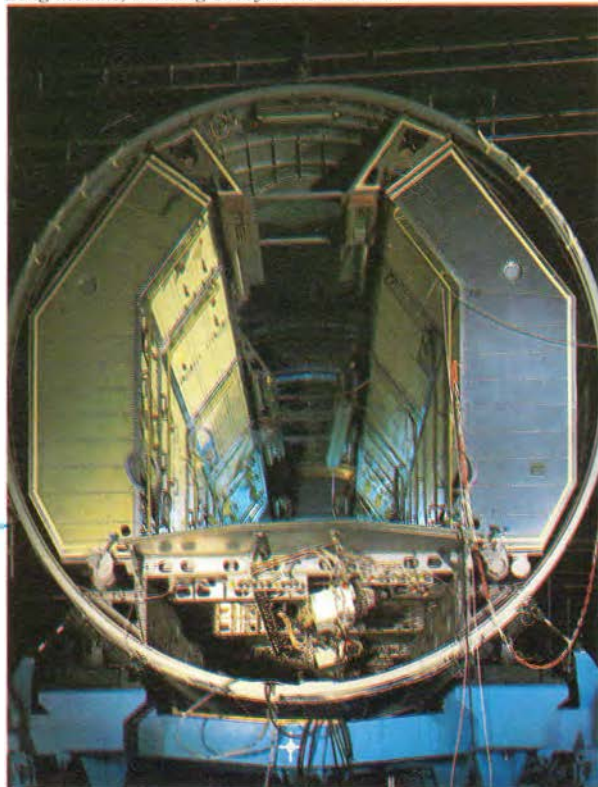
Long module, showing subsystems and racks
