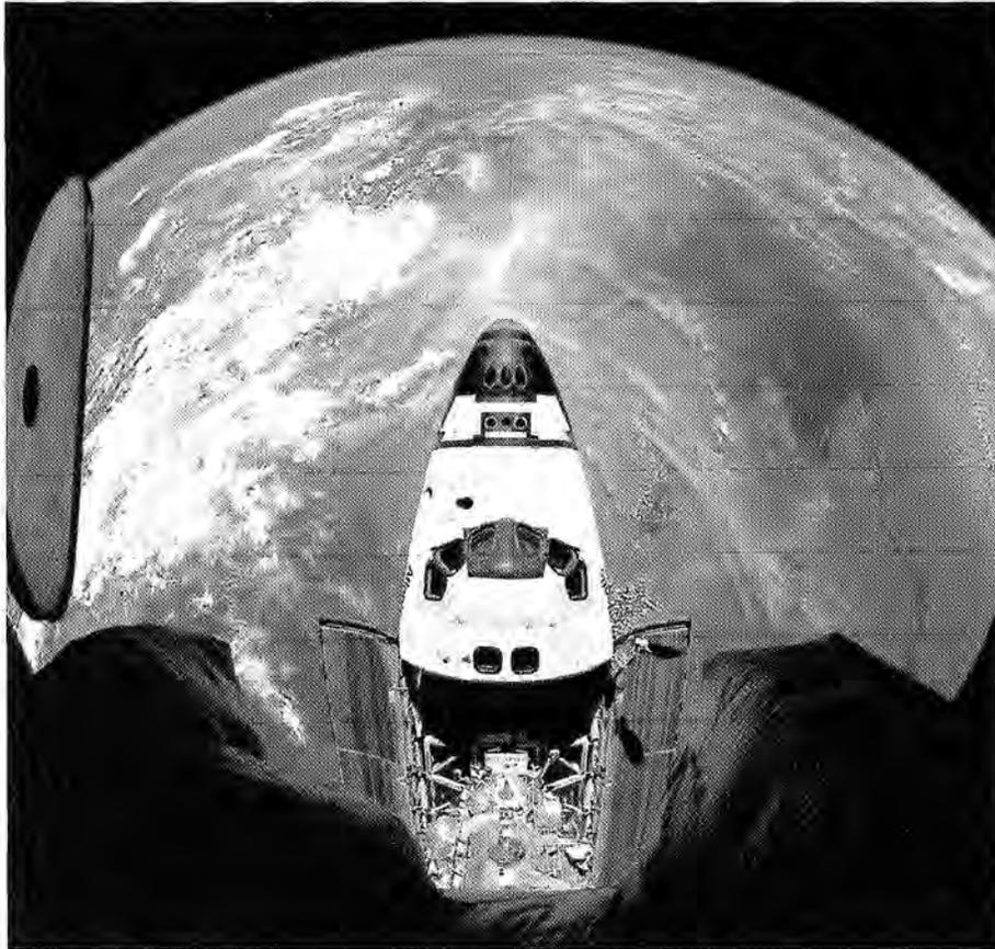
The Space Shuttle cannot be flown without a human pilot; it is the first piloted spacecraft of the United States that has no capability for automated flight. This fisheye view of the Space Shuttle *Atlantis* is seen from the Russian *Mir* space station during the STS-71 mission. (NASA photo no. STS071-741-004)
