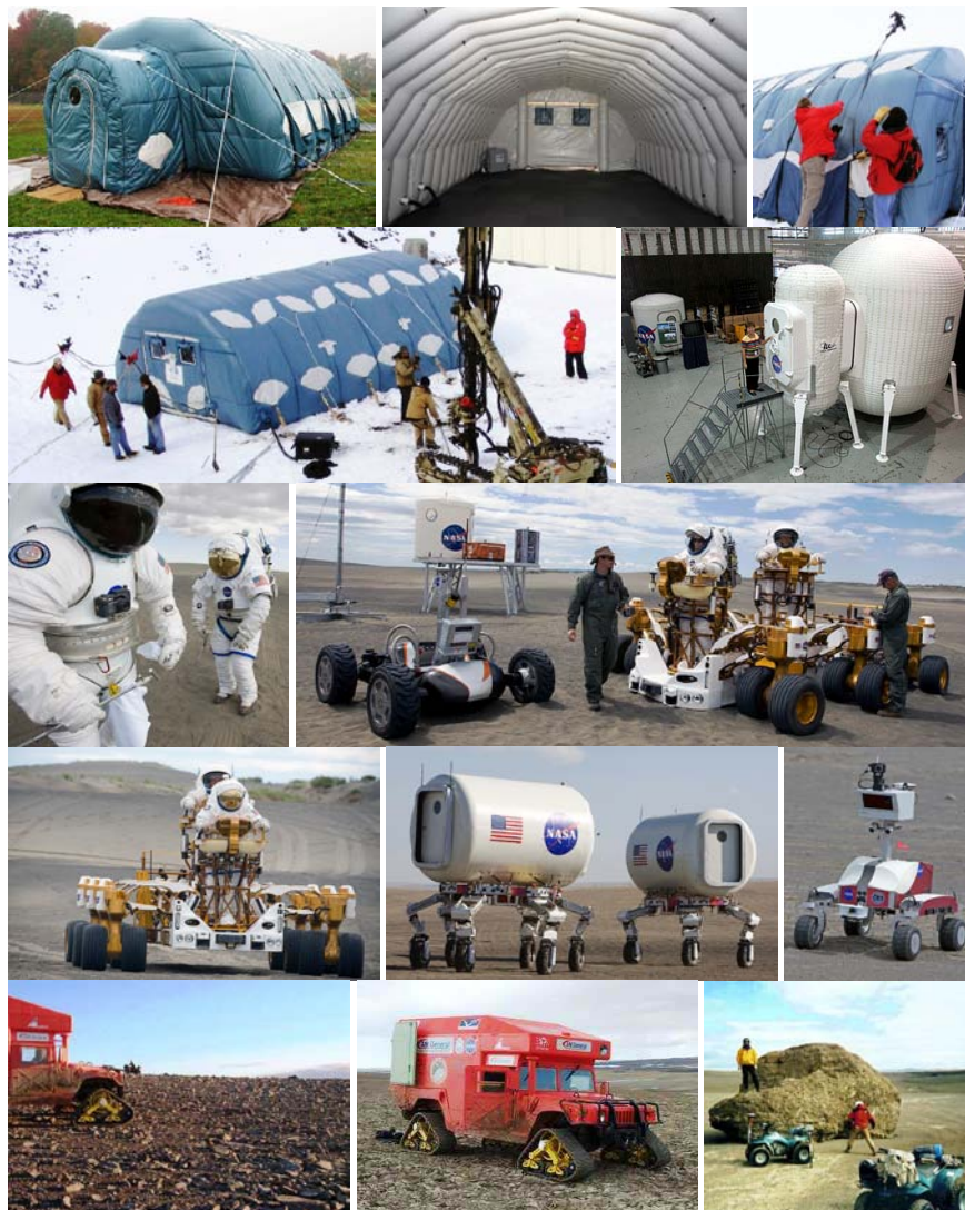
Figure 1-5: Prototype inflatable lunar habitats are tested in the Antarctic. Surface suits and a new rover concept vehicle, along with mobile lunar habitats and scout robots, are tested at Moses Lake in Washington. An experimental Humvee rover and all-terrain scout vehicles are used to test planetary surface navigation techniques (a 230 kilometer trek using only satellite imagery and topography data) on the Mars-like polar desert terrain of Devon Island inside the Arctic Circle.
