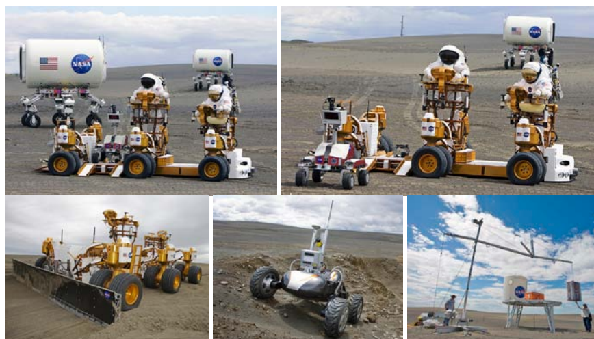
Figure 2-13. With mobile lunar habitat modules in the background, astronauts on a “lunar truck” deploy a robot scout rover. The lunar truck doubles as a bulldozer. An automated drilling unit makes its way over simulated lunar terrain. An electric crane is tested for removing equipment from a simulated lunar lander.
